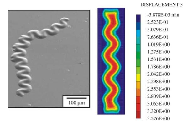
In the above figure, the “telephone cable” delamination of a thin film on a substrate is shown.
